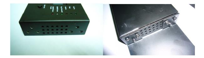
Then install the mounting brackets onto both sides of the controller. Please refer to the diagrams above. After that the controller can be mounted in a 19" rack as below:
